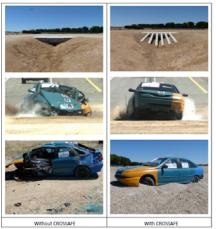
✓ Modular: Adaptable to any type of ditches, independently of the geometric and structural characteristics, since different elements can be assembled to cover wider ditches.
