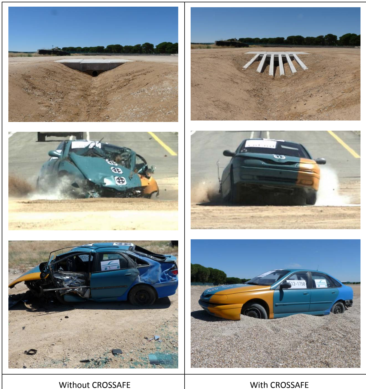
Figure 14.- Car crash test with a mass of 1500 kg, a speed of 100 and an angle of 0°, without and with culvert-end protection system Crossafe
